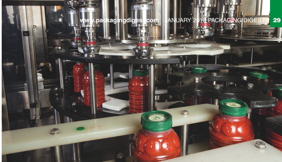
Filled bottles exit the capper, above, and head to the labeler, which applies a one-piece wraparound label without having to be oriented, improving line efficiency and enhancing the label billboard space.
