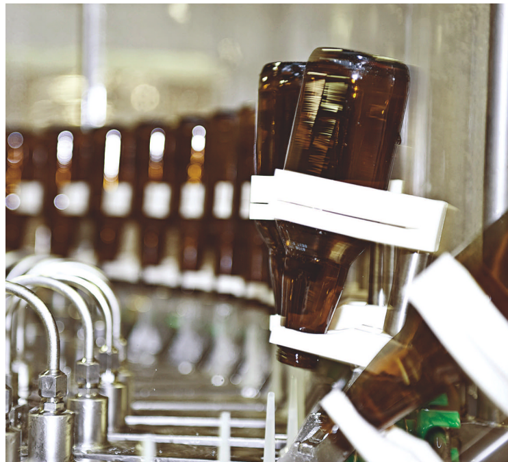
After being washed in a 60-valve rinser, bottles enter a 78-valve filler, top. The last item in the monobloc system is a 13-head crowner. Rinsing solution discharges from the inverted bottles in the rinser, below.
