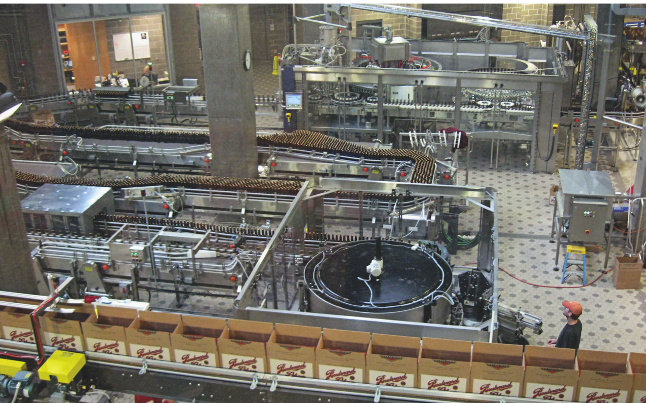
Left, view of the second-floor equipment looking from the labeler (bottom) to the rinser/filler/crowner (top). Note the varying bottle density on the conveyors as they go from bulk transport to single filling. The three-station labeler, above, applies front, back and neck labels. An inspection unit after the filler checks the fill level in the bottles.
