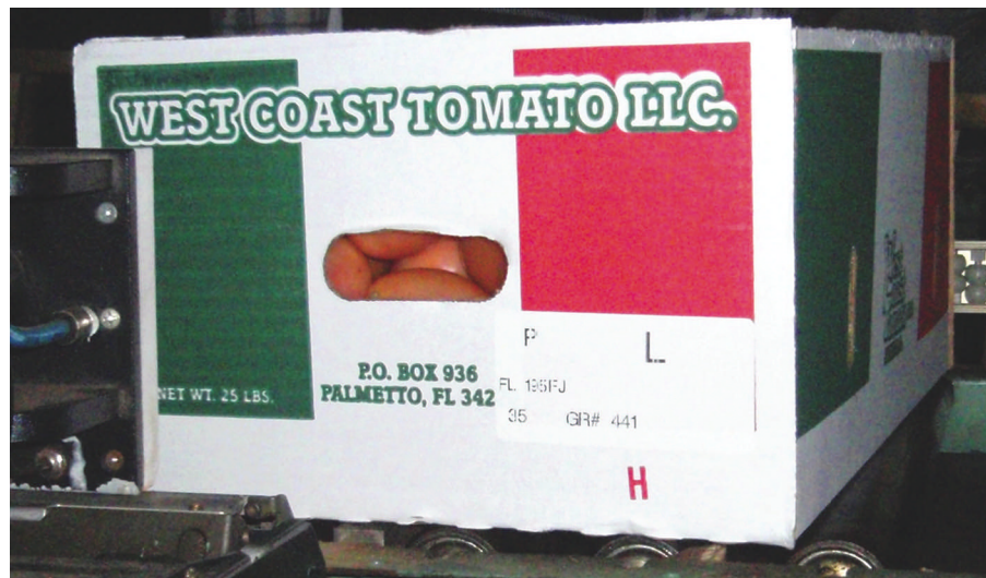
Two different automated fillers, each handling a different type of tomato, feed 25-lb cases of fruit to each line. As those cases merge, photoelectric eyes trigger the print/apply system to produce the correct label, depending on which filler the case came from, and apply it as the case moves down the conveyor.
