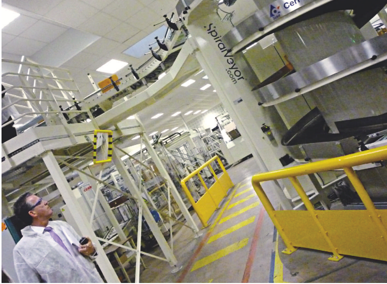
Pallets travel up a spiral conveyor in preparation for palletization. The end-of-line system's two-level layout enables it to fit between a wall and another line.
