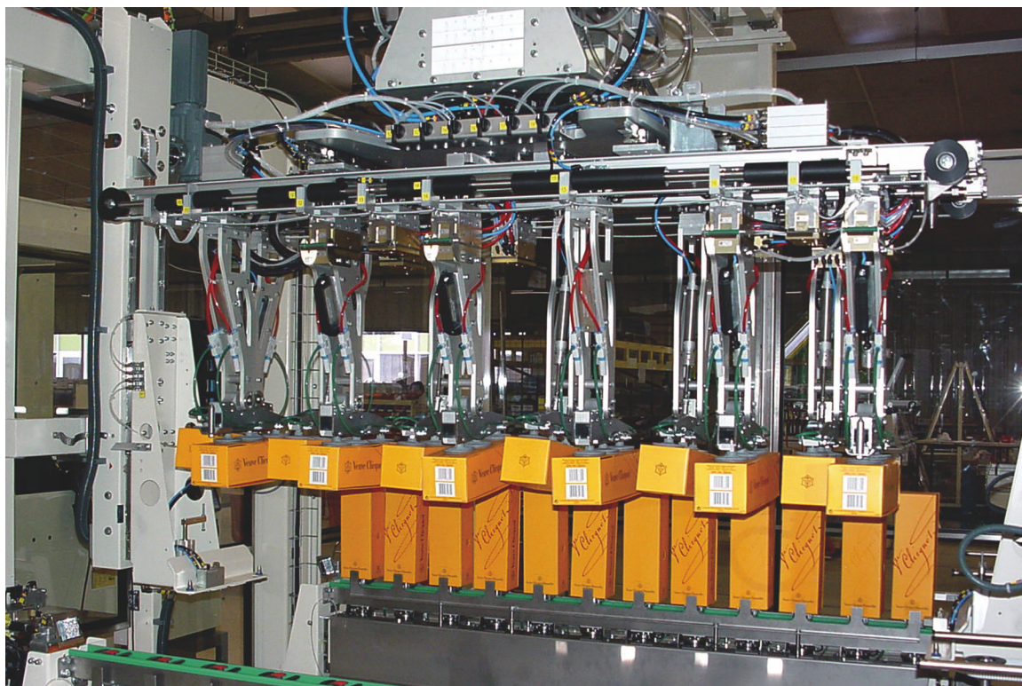
The two-axis AN110 gantry packer is a multi-function machine with a payload of 250 kg (products and tooling). The AN110 packer, above, orients Veuve Clicquot DesignBoxes for proper facing.
