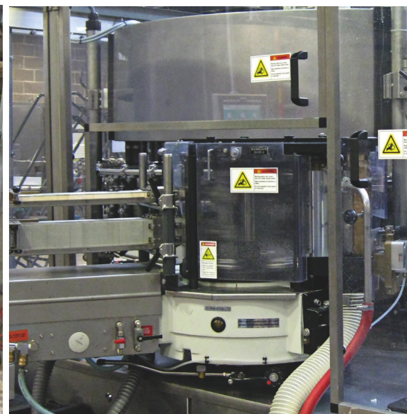
Left, view of the second-floor equipment looking from the labeler (bottom) to the rinser/filler/crowner (top). Note the varying bottle density on the conveyors as they go from bulk transport to single filling. The three-station labeler, above, applies front, back and neck labels. An inspection unit after the filler checks the fill level in the bottles.
