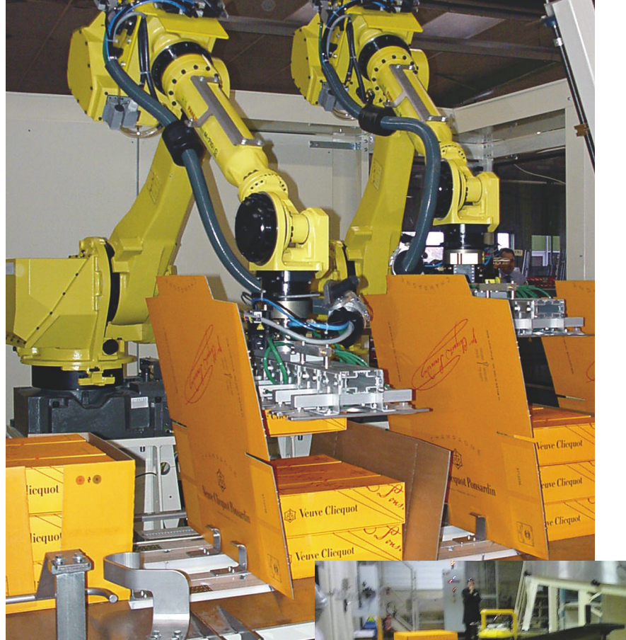
Two robots, integrated in the WB45.80 case packer, place oriented DesignBoxes into wraparound cases, above. A print-and-apply labeler, right, places a bar-coded label onto one side of a sealed wraparound case.
